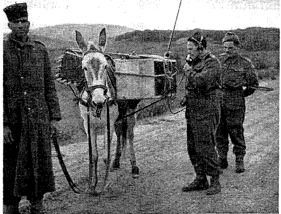
MULE-BACK RADIO. An unusual mounting for a transmitter-receiver seen in N. Africa, where Arab muleteers have been recruited to assist our Forces.
